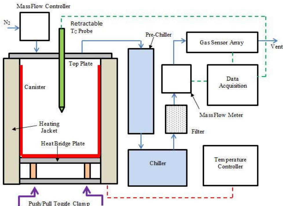
Figure 1. Schematic of the full-scale prototype TPU.<sup>11,18</sup>
