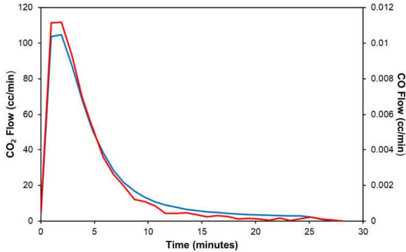
**Figure 5.** CO (red) and CO<sub>2</sub> (blue) flows measured after the initial 48 hour storage period at room temperature, for 210 g of human solid waste. The total yields for CO and CO<sub>2</sub> were 0.57 cc and 598 cc, respectively.
