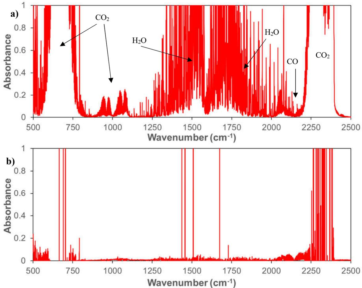
**Figure 6.** Infrared absorbance spectrum obtained for human solid waste decomposition gas after a storage period of ~48 hours: (a) shows the uncorrected data, dominated by CO<sub>2</sub> and H<sub>2</sub>O features; (b) shows the data with CO<sub>2</sub> and H<sub>2</sub>O interferences removed and the CO band in the region between 2000 and 2300 cm<sup>-1</sup> is more apparent. An expanded view of the CO band appears in Figure 7.
