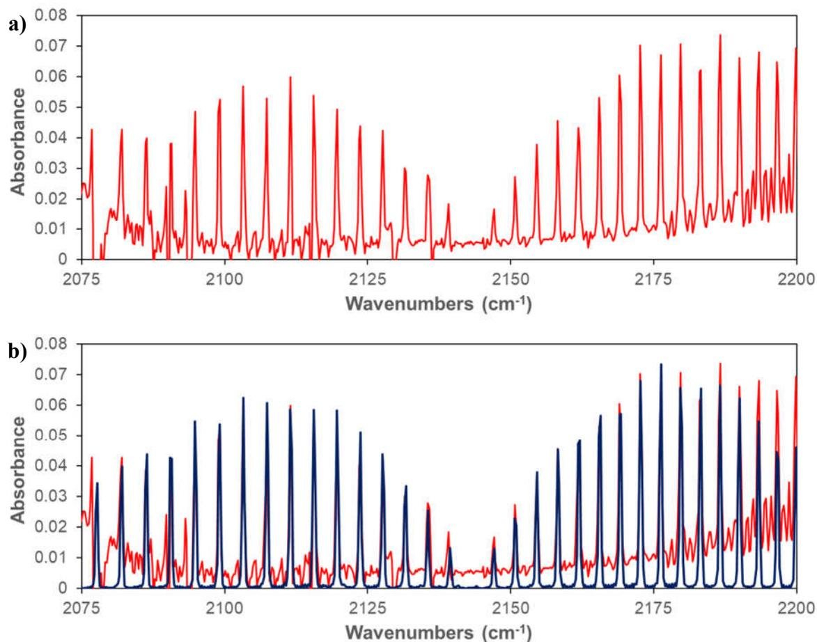
**Figure 7. Infrared absorbance spectrum measured for human solid waste decomposition gas (red) after a storage period of ~ 48 hours: (a) spectrum is the same corrected data shown in Figure 6b but zoomed in on the CO band region; (b) plot shows the measurement overlaid with a 30 ppm CO calibration spectrum (blue).**
