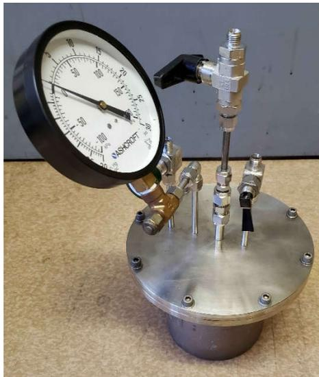
**Figure 4. Reaction canister used for stored human solid waste gas evolution testing.**
