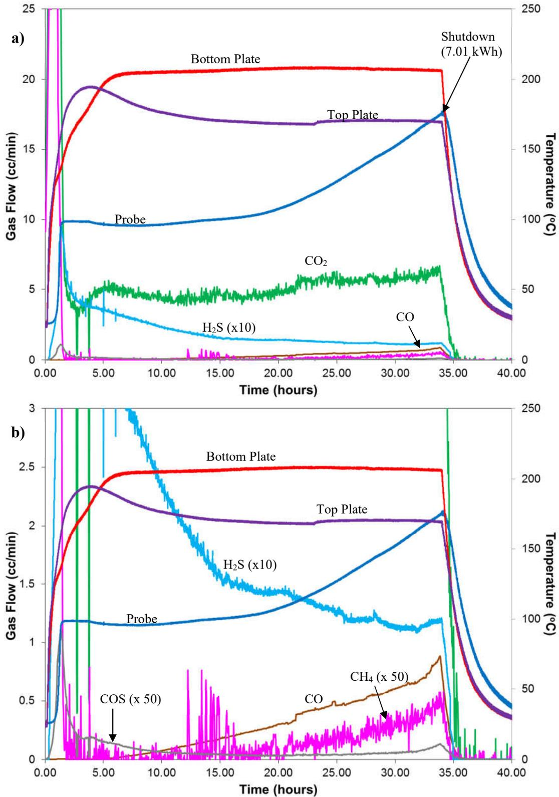
**Figure 2. (a) Temperature and gas profiles recorded during a full-scale TPU test with human solid waste for Run # 329; (b) Plot is zoomed in at lower gas flows to highlight the trace gas profiles. The wall setpoint temperature was ~205 °C and the target endpoint at the center was 175 °C.**
