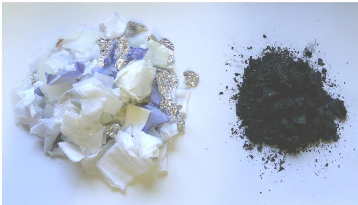
**Figure 10.** Photograph of a typical HFWS sample before and after microwave pyrolysis.
