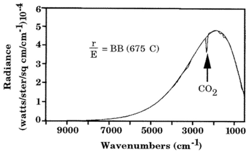
**Figure 5.** Determination of Temperature by Matching ( $r/E$ ) with a Blackbody Curve.
