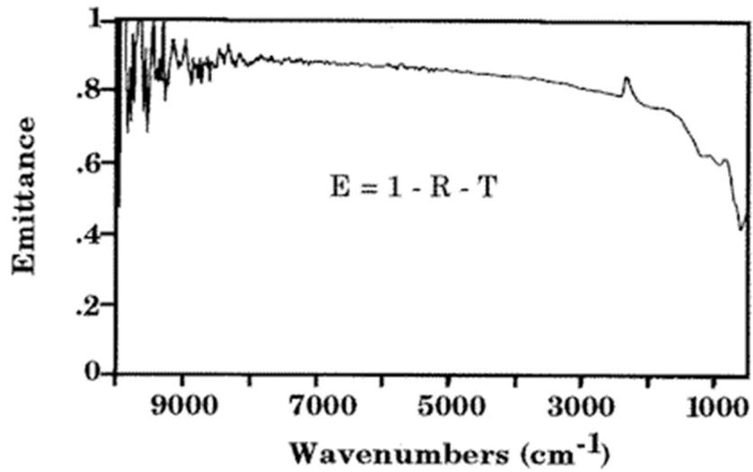
**Figure 4.** Determination of Spectral Emittance from the Measured Hemispherical Reflectance ( $R$ ) and Hemispherical Transmittance ( $T$ ).
