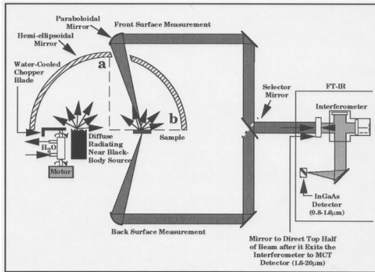
**Figure 2. Schematic of Benchtop Emissometer.**
