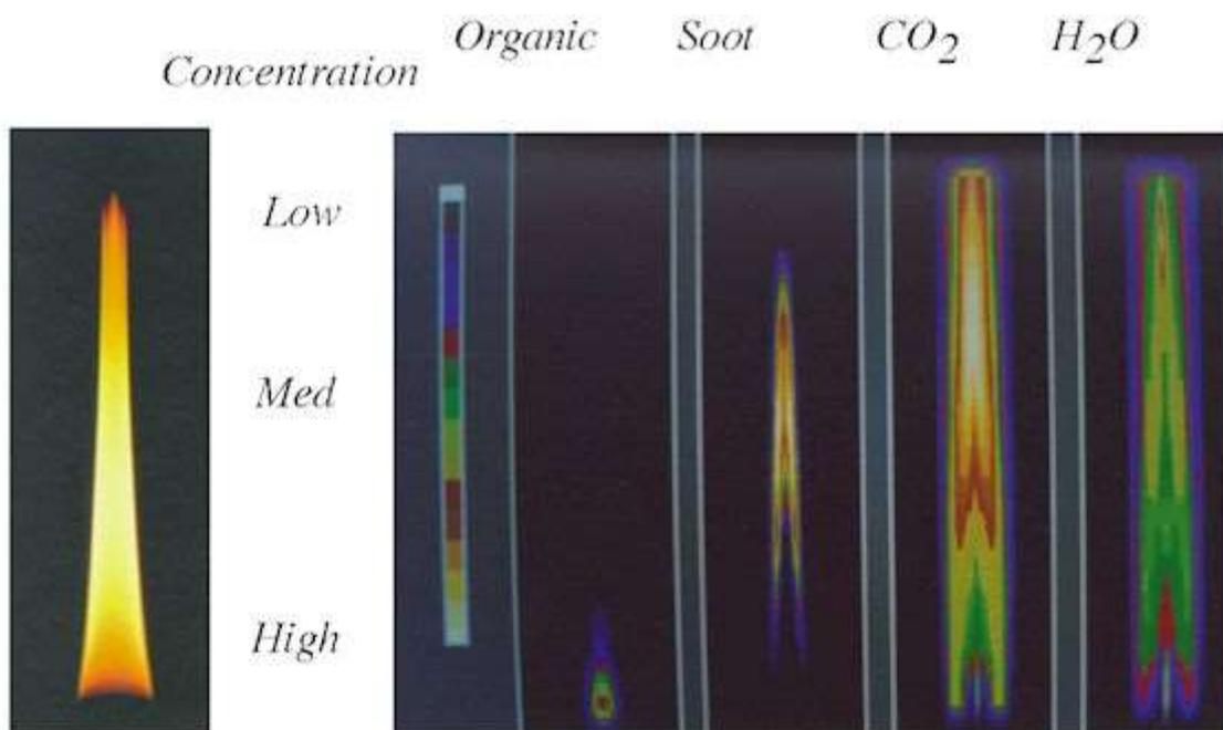
**Figure 3.** The Ethylene Diffusion Flame with Central Plane Images of Relative Concentration Reconstructed from FT-IR Transmission.
