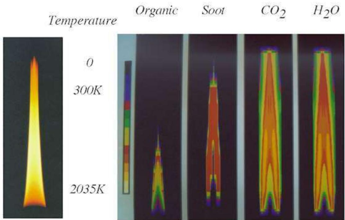
**Figure 4.** Central Plane Images of Temperature Reconstructed from FT-IR Transmission and Radiance Spectra.
