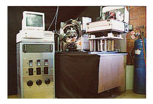
Figure 1. Series 205 Spectral Emissometer.
