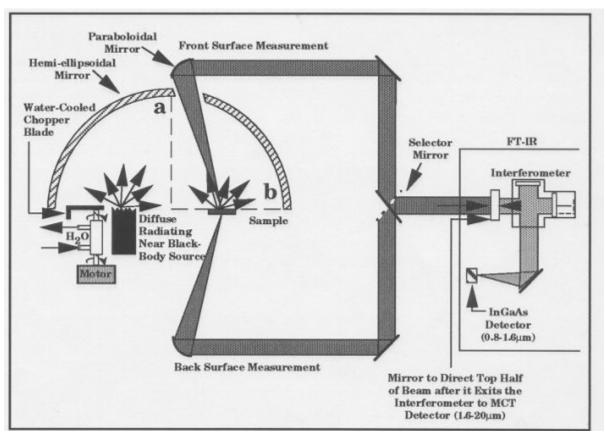
Figure 2. Schematic of Benchtop Emissometer.
