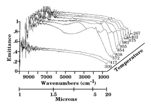
**Figure 6**. The Radiative Property Change of a Metal Alloy as it is Heated in Air.
